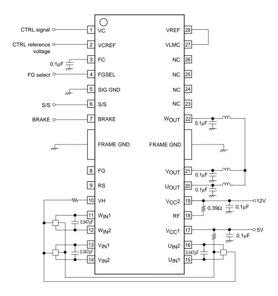
The values of the capacitors between power supply and ground, between output and ground, and between the Hall sensor inputs vary depending on the motor used. In particular, the Hall sensor input capacitors may not be required for some motors.
