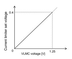
The LB11699H current limiter set voltage is the VLMC pin voltage, and varies as shown in the figure to the left. When the VLMC pin voltage is 0V, the current limiter set voltage will be 0V and no output current will flow.
